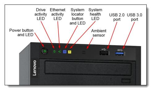
Figure 19. Front operator panel
