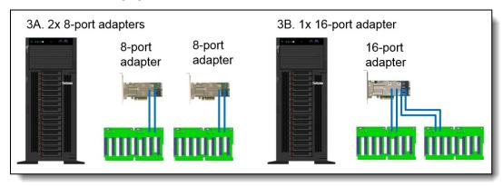
Figure 9. Adapter and cabling for 16 drive bays, all SAS/SATA
