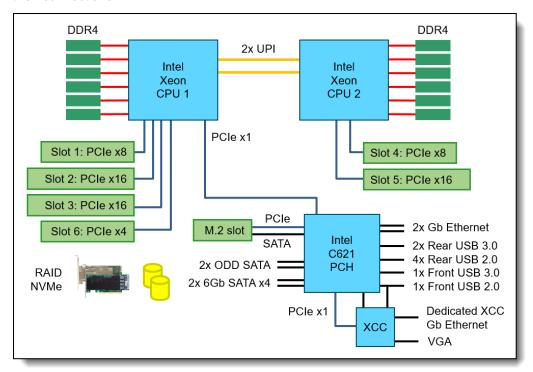
Figure 5. ST550 system architectural block diagram
