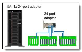
Figure 11. Adapter and cabling for 20 drive bays, all SAS/SATA
