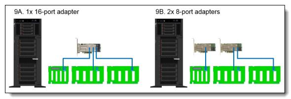
Figure 15. Adapter and cabling for 8x 3.5-inch + 4x 2.5-inch drive bays, all SAS/SATA
